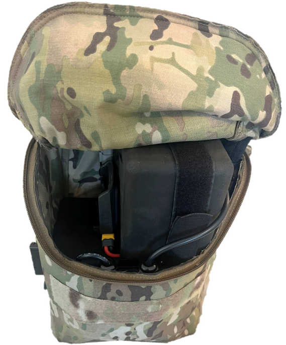
Receiver fully integrated within power unit
